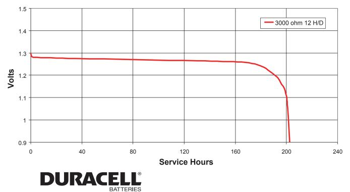
\* Delivered capacity is dependent on the applied load, operating temperature and cut-off voltage. Please refer to the chart and discharge data shown for examples of the energy / service life that the battery will provide.
